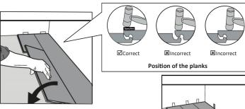
place it tight to the short end of the previous plank with an angle of 30 degrees. Lower the plank until it is resting in line with the adjacent plank. Firmly strike the surface of the locking mechanism with a Soft Faced Hammer and a tapping block until the planks are locked together at the same height. Make sure both planks are  $\,$
