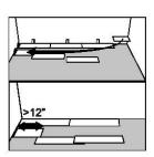
⑥ Start the second row with the leftover cut part of the last plank of the previous row. This small plank should measure at least 12". Otherwise, use another plank that should be cut in two. The end joints of each adjoining row should not be closer
