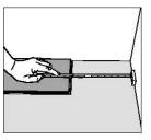
4 At the end of the first row, leave an expansion gap of 1/4" to the wall and measure the length of the last plank to fit.
