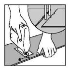
$\ensuremath{ \textcircled{\scriptsize 11}}$  Holes for pipes: measure the diameter of the pipe and drill a hole that is ¾" larger. Saw off a piece as shown in the figure and lay the board in place on the floor. Then lay the sawed-off
