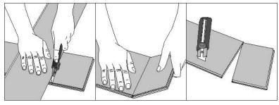
(5) To cut the plank, use a simple utility knife and ruler, and with the top side facing up, cut heavily and several times on the same axis. The knife will not go through the surface but make a deep cut. You can then lift one half of the plank using your other hand to hold down the second placing it very close to the cut. The plank will split naturally.
